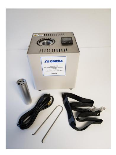
Above items are included with the DBCL400 Dry Block temperature calibrator. Not shown is the calibration certificate and operator manual
